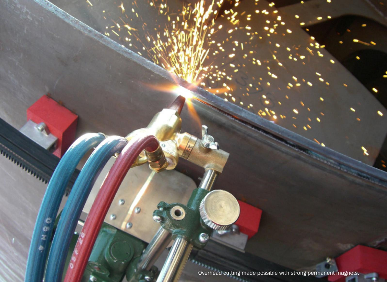
Overhead cutting made possible with strong permanent magnets.
