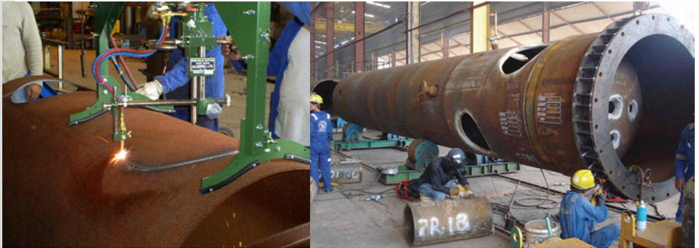
The KHC-600D is ideally suited for cutting high precision T- joint circles including any hole that crosses the side of the pipe for piping systems, high pressure vessels and heat exchangers. Developed with KOIKE Advanced Technology, the KHC-600D is a compact design that is light weight and easy to operate. In addition to cutting circles and bevel in flat plate, the machine can cut holes in vessels from the inside or outside.
