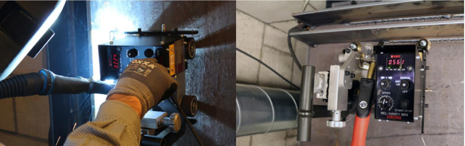
The Wel-Handy Mini Strong is a compact design welding carriage designed to perform horizontal, vertical, and overhang welding. A 35 kg magnet and 16 kg traction power provides reliable performance and quality welds. The machine is easily carried around with the handle with magnet detachment mechanism.
