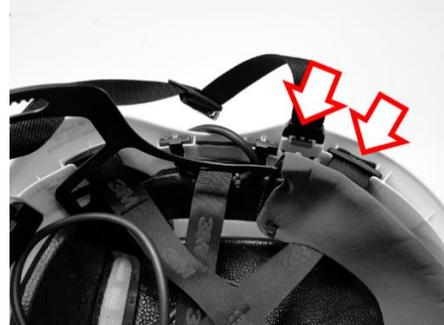
4. Cut the cable tie. Re-attach the head harness and strap on the helmet.
