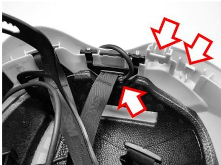
3. Detach the head harness and strap from two points on each side of the helmet. Attach the cable at the mark to the harness with the cable ties.
