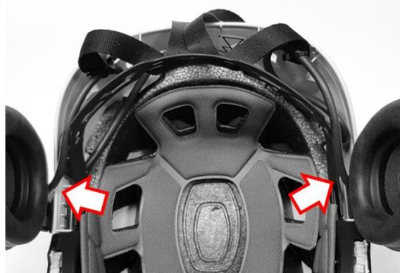
4. Check that the cable can move freely when earmuffs are moved between parking and standby position.
