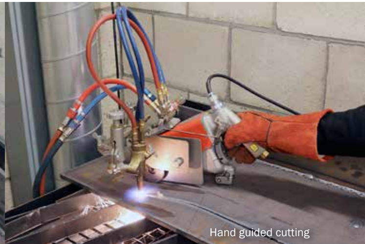
Straight cutting with IK-93 rail
